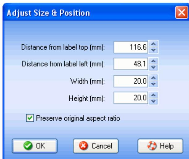
This dialog lets you change the size, position, and aspect-ratio preservation of an image you've added to a label. All units in this dialog are in millimeters.
